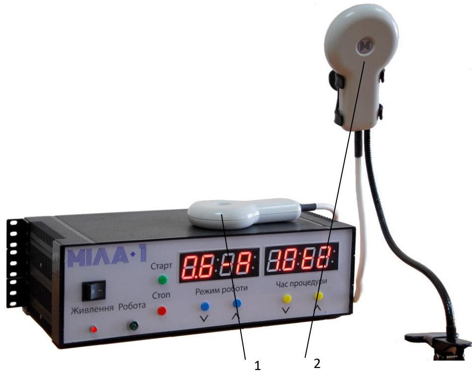
Figure 2. The apparatus with inductors: 1 - No 1 inductor (indicated by 1 on the housing of the inductor); 2 - No 2 inductor (indicated by 2 on the housing of the inductor).
