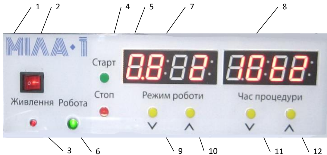
Figure 1. The front panel of the apparatus: 1 - the name of the apparatus; 2 - power switch; 3 - LED power switch; 4 - Start button; 5 - Stop button; 6 - Work indicator; 7 - digital indicator of the selected treatment procedure; 8 - digital indicator of the selected time of the treatment procedure; 9 – “down” button for selecting the procedure mode; 10 – “up” button for selecting the procedure mode; 11 - “down” button for setting the time of the procedure; 12 - “up” button for setting the time of the procedure.
